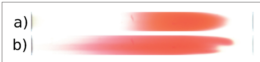
Figure 3a and b. The photographs illustrate the change in shape of elution bands as a function of the viscosity contrast. The refractive index system was matched with the stationary phase, so that the column becomes transparent. In both cases the viscosity of the injection plug was 0.38 cP. The injection volume was 5 µL and the flow rate was 0.5 mL/min. Flow direction is from left to right. In (a) mobile phase viscosity 0.38 cP, i.e. viscosity contrast around 0 and in (b) mobile phase viscosity 1.44 cP, i.e. viscosity contrast about 3.8 times. The figure was adapted from Figure 7a and b in [10].
