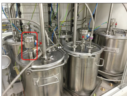
Figure 4: Fraction collection containers located inside a dedicated fume hood. The solvent level sensor (highlighted) is fitted to each container to prevent overflowing.
