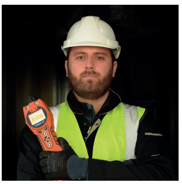
Concentration of target chemical = isobutylene calibrated measurement x RF
