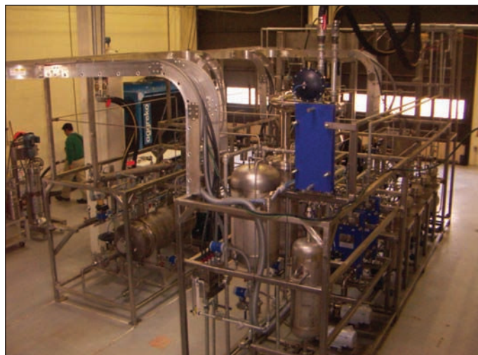
Fig. 4: Pilot scale SFC at Malaysian Palm Oil Board: 350mm I.D. column, 600 kg CO 2 /hr (max), Co-solvent pump : 40 L Co-solvent/hr (max) [Ng, 2008]
