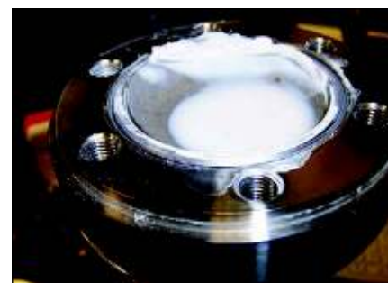
Figure 3. Result of Inlet Frit Blockage and Consequent Over-pressure in an SFC Column. CHIRALPAK AD-H, 250 x 50 mm.
