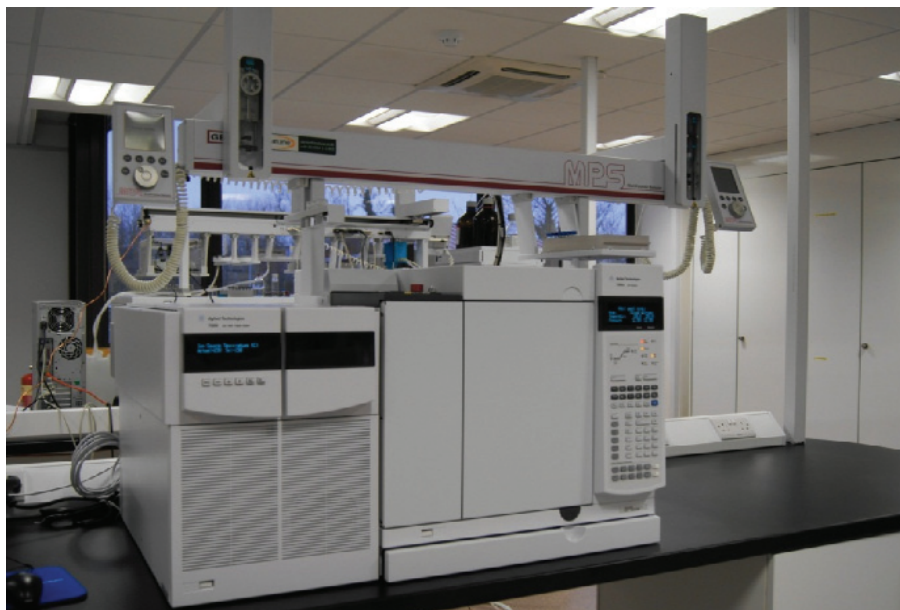
Figure 2. An Agilent GC 7890A GC and 7000 MS triple Quad with MPS 2 XL (Dual Head) CIS Multiflex Inlet used to determine environmental pollutants in water. Picture courtesy of Anature Ltd.
