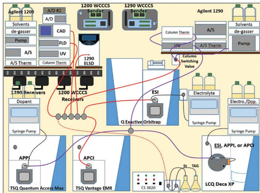
Figure 1: Arrangement of instruments for LC1MS2 x LC1MS2 = LC2MS4 experiments. <sup>1</sup>D: Agilent 1200 quaternary HPLC with UV, FLD, CAD, ELSD, HPLC ESI-MS, and APCI-MS; <sup>2</sup>D: Agilent 1290 binary UHPLC with UV, APPI-MS and ESI-MS. Controlled by wireless communication contact closure system (WCCCS).
