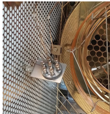
Figure 4: Schematic (Left) and photo (Right) of the RFF valve-based INSIGHT modulator for GCxGC. In fill mode, the primary column eluate enters the sample loop (with any overflow directed to a bleed line), while the modulation valve directs auxiliary carrier gas to the secondary column. The valve switches and the contents of the sample loop are flushed rapidly onto the secondary column as a narrow band. Image courtesy of SepSolve.
