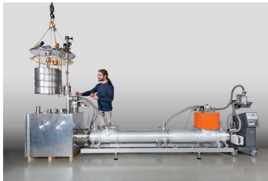
SuperSun - a new high-density source for ultracold neutrons Credit: Laurent Thion ILL
