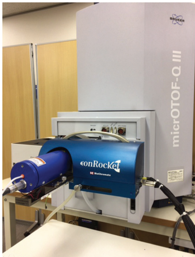
Figure 1b. ionRocket coupled with DART placed directly on the Mass Spectrometer front end.
