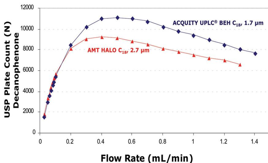
Figure 2: Efficiency vs. flow rate curves for 2.1 x 50mm columns. The analyte is decanophenone, the mobile phase is a mixture of acetonitrile and water (70/30, v/v), the temperature is 30°C and the system is an ACQUITY UPLC with a TUV detector. Efficiencies were corrected for system dispersion.
