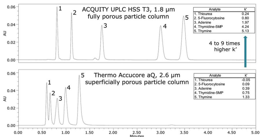
Figure 8. Comparison of retention factors for two 2.1 x 50mm reversed-phase columns designed to retain polar compounds using highly aqueous mobile phases. Note the increased retention factors ( $k'$ ) for the fully porous particle ACQUITY UPLC HSS T3 column (top). The mobile phase is 10mM ammonium formate, pH 3.0, the flow rate is 0.2mL/min, the temperature is 30°C and the system is an ACQUITY UPLC with a TUve detector (set to 254nm).
