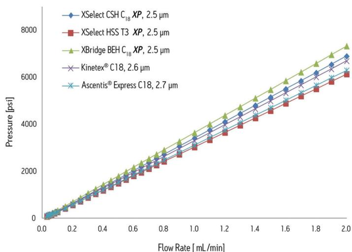
Figure 3: Backpressure vs. flow rate for five 2.1 x 50mm columns. The mobile phase is a mixture of acetonitrile and water (75/25, v/v), the temperature is 30°C and the system is an ACQUITY UPLC with a TUV detector. Pressure values were corrected for system backpressure.
