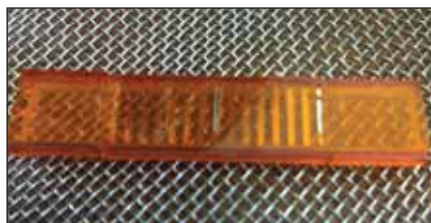
Figure 5. PMMA Sputtering mask for Platinum PVD.
