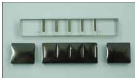
Figure 6. PMMA mask post platinum PVD, platinum electrodes formed on glass chip.
