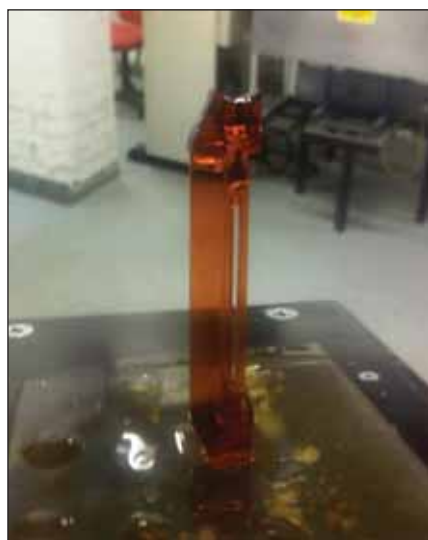
Figure 7. Replacement component manufactured using stereolithography RP. Channel widths ranged from 1 mm down to 100 \mu m.
