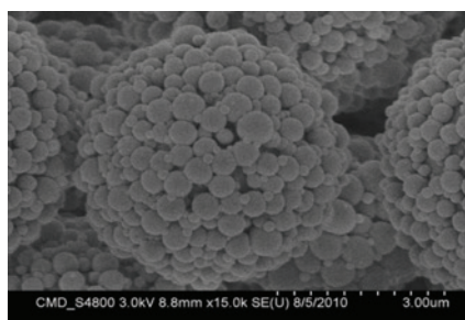
Figure 3 Potential fractal structure starting to appear with spheres on spheres on spheres of solid silica
