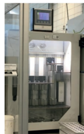
Figure 5: 'Bespoke' Reverse phase purification system column oven supplied by ABSys.
