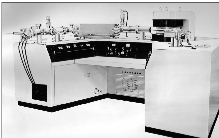
Figure 1: Picture of the Hitachi PerkinElmer, model HMR-2 high resolution mass spectrometer, used for LC-MS interfacing development at Cornell University (by courtesy of Professor Fred McLafferty, 2012).
