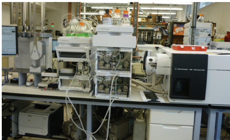
Figure 1. An example of a 2D UHPLC MS/MS system utilising UHPLC pumps in both dimensions.
