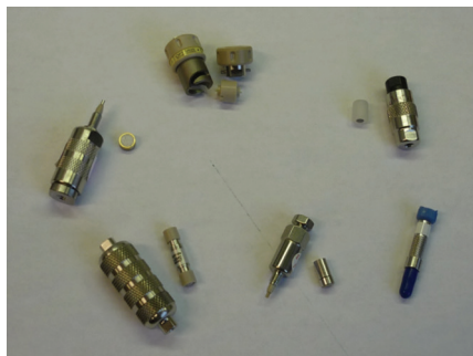
Figure 2. Different guard cartridges and trap columns available for on-line analyte trapping.
