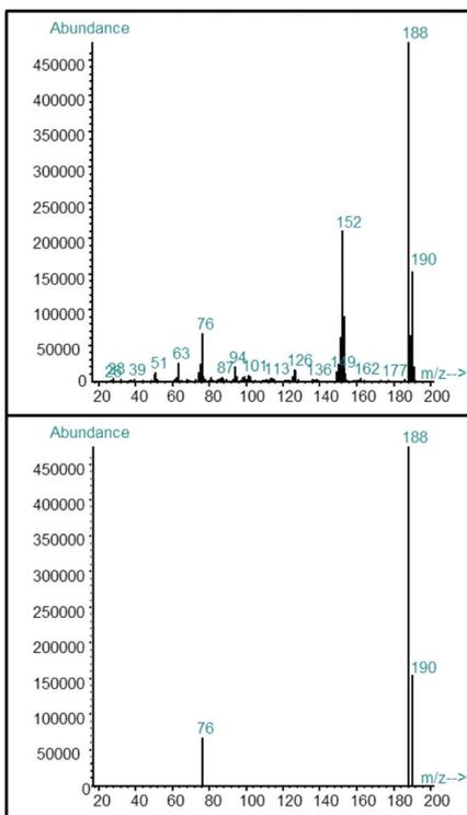
Diagram 7: SIM has less noise and allows more ions of the m/z range through to the MS detector therefore giving higher sensitivity than SCAN
