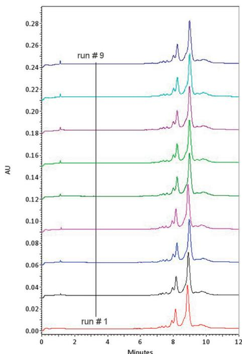
Figure 4: CZE separation of MAb X. Nine consecutive separations of MAb X were performed using UV detection. MAb X concentration was 1mg/mL; separation buffer: 0.05% HPMC, 380 mM EACA, 1.9mM TETA; bare fused silica capillary, 30 kV separation voltage.
