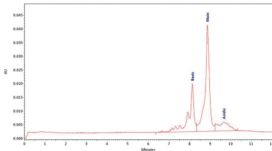
Figure 2: CZE profile and peak integration strategy for MAb X. Peaks were grouped as either Basic, Main or Acidic variants. CZE conditions: MAb X 1mg/mL; Separation buffer: 0.05% HPMC, 380 mM EACA (epsilon amino caproic acid), 1.9 mM TETA; bare fused silica capillary, 30 kV separation voltage.
