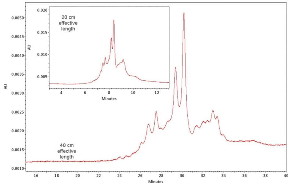
Figure 7: MAb X degraded by exposure to high temperature (60°C) for 5 days. CZE separations were performed as described previously using either 40cm capillary (bottom trace) or a 20cm capillary (inset).
