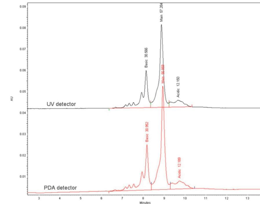
Figure 5: Comparison of UV and PDA in CZE separation of MAb X. CZE was performed using either UV detection (red trace) or PDA detection (black trace). Separation conditions are the same as those described in Figure 1.
