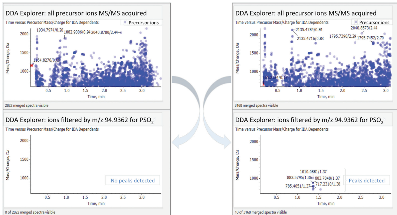
Figure 4: DDA Explorer (time versus precursor MS/charge for DDA dependents) and DDA Explorer filtered by m/z 94.936 with 10 ppm mass tolerance of deproteinated plasma with 4.5 \mu\text{g/mL} oligo dT (blank sample), and with 10 ppm mass tolerance of 100 ng/mL PSOs in deproteinated plasma with 4.5 \mu\text{g/mL} oligo dT (spiked sample).
